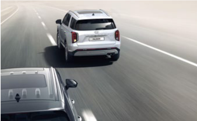
Forward Collision-Avoidance Assist (FCA) If the preceding vehicle suddenly slows down, or if a forward collision risk is detected, such as a stopped vehicle, a pedestrian or a cyclist in front, it provides a warning. After the warning, if the risk of collision increases, it automatically assists with emergency braking. Blind Spot Collision Warning (BCW) When operating the turn signal switch to change lanes, if there is a risk of collision with a rear side vehicle, it provides a warning. If exiting a parallel parking spot and there is a risk of collision with a rear side vehicle, it automatically assists with emergency braking.
