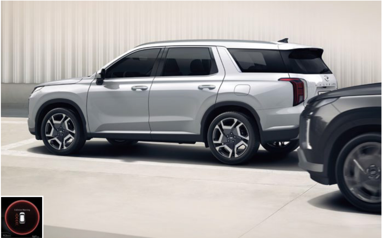
Safe Exit Assist (SEA) When the occupant opens the door to exit the vehicle after a stop, if an approaching vehicle from the rear side is detected, it provides a warning. It also helps keep the rear door closed through operation of the electronic child lock.
