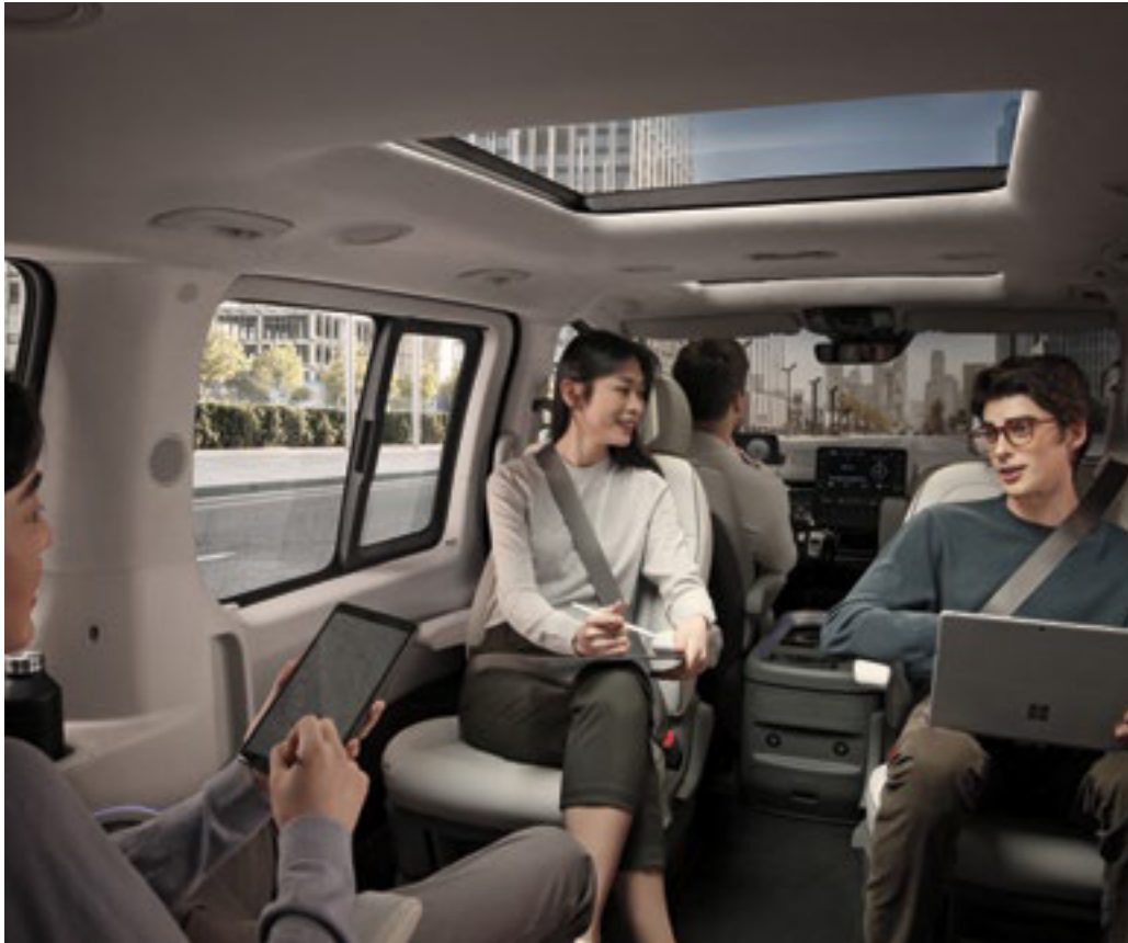
Swiveling independent seat STARIA Premium's flexible seating multiplies the fun factor, especially when traveling with children on long-distance trips. The 2nd-row swiveling independent seat rotates 180° degrees to allow face-to-face conversation among rear seat passengers and 90° to promote easier entry and egress.
